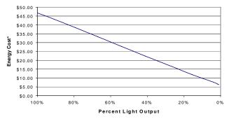
\*Energy Cost based on 4000 hrs./yr. Operation @ \$0.10 kWh
