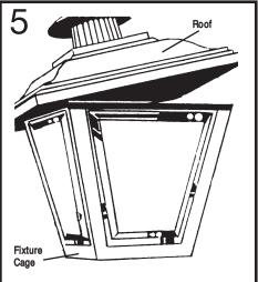
SCREW LIGHT BULB INTO SOCKET. Be sure to use bulb with wattage no greater than specified for this fixture. Lower roof and snap into place.
