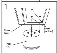
FASTEN THE CAGE to the post cup with the 3 screws provided.
