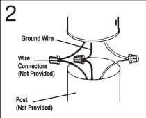
CONNECT THE WIRES. NOTE: Attach black fixture wire to black supply wire, white fixture wire to white supply wire. Do not mix them up. Use approved electrical tape or wire connectors (not provided). Connect bare fixture ground wire to ground wire from outlet box. NEVER CONNECT GROUND WIRE TO BLACK OR WHITE POWER SUPPLY WIRES.
