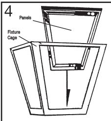
INSTALL PLASTIC PANELS, textured or beveled side out, by sliding panels down cage in slots on inside of cage. Make sure panels are all the way down into seats in cage
