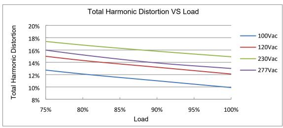
Note: The above data is derived from the MSPI-DIM70W12S-1750 test.
