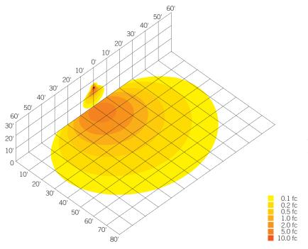
Ground mounted at 6" above ground, 10° above horizontal, shining towards building exterior
