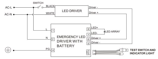
1.DO NOT MATE CONNECTOR UNTIL INSTALLATION IS COMPLETE AND AC POWER IS SUPPLIED. 2.TEST ACCESSORY LEADS-OBSERVE PROPER POLARITY WIRING.
